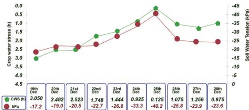
Figure One: 'Crop water stress' versus average soil moisture tension for a one-week period: when irrigation was withheld. The steady increase in crop water stress corresponds well with the increasingly dry soil conditions
