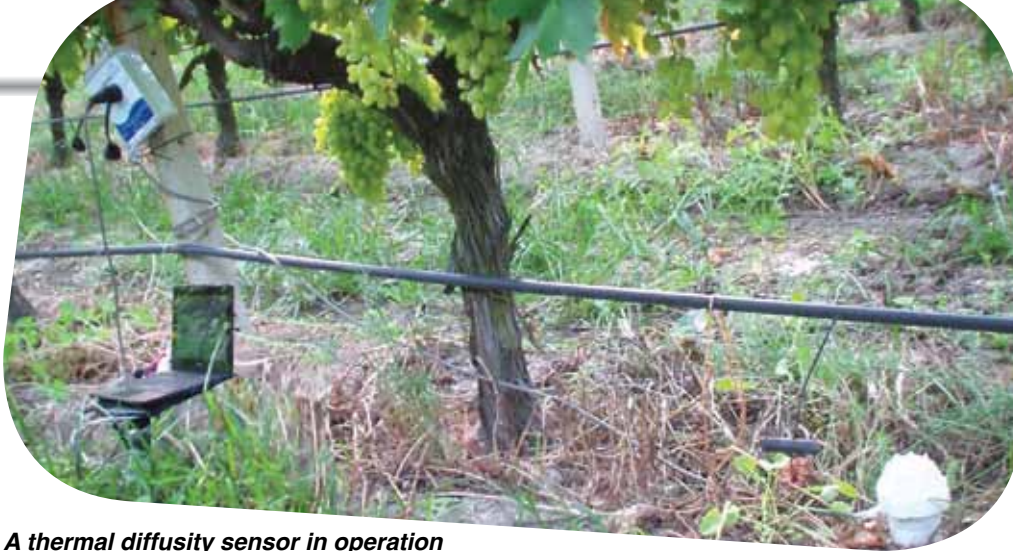
A thermal diffusivity sensor in operation
